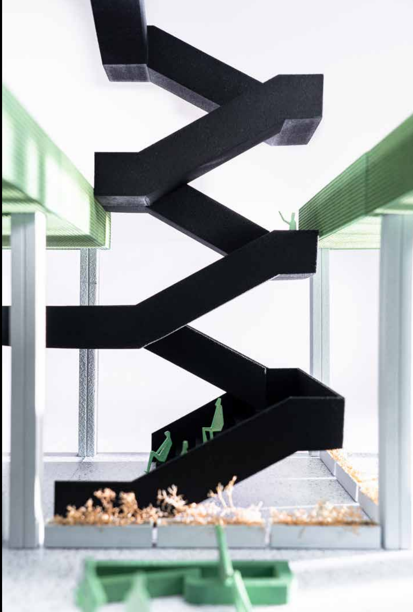
3D-printed study into helix-like access stairs VRT building, Brussels — VRT
